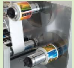
Rewinding to finished rolls
